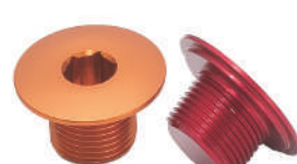
CC-CHB02 For SRAM MTB ■ Material AL7075T6 ■ Length M15 25.8X12.8Lmm ■ Finish Anodized Color
