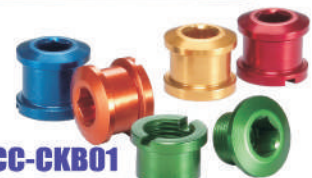
CC-CKB01 ■ Material AL7075T6 ■ Length M8-0.75X6.5L For Road M8-0.75X8.5L For MTB ■ Finish Anodized Color
